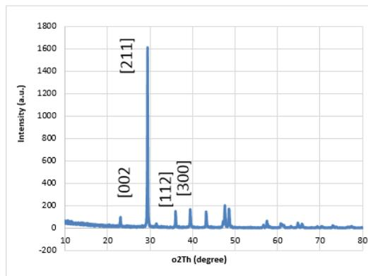
Fig. 2. Phase Identification of Eggshell Nanopowder without Sintering at 1100°C
