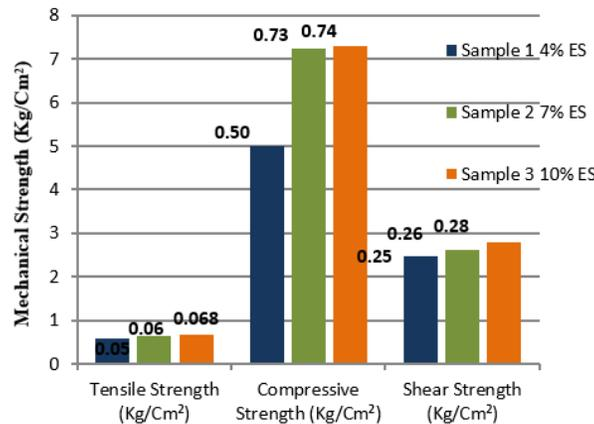
Fig. 3. Mechanical Properties of Sand Moulds in Wet Conditions
