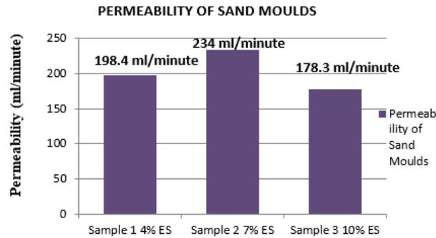
Fig. 5. Results of Permeability Testing on Sand Moulds
